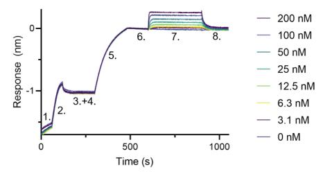
BLI binding kinetics of a mouse IgG1 anti-DYKDDDDK-tag antibody to a DYKDDDDK-tagged protein. A monoclonal mouse IgG1 anti-DYKDDDDK-tag antibody was immobilized using Nano-CaptureLigand mouse IgG1, Fc-specific VHH, biotinylated on FortéBio Streptavidin (SA) Biosensors and assayed with different concentrations of a DYKDDDDK-tagged protein.
