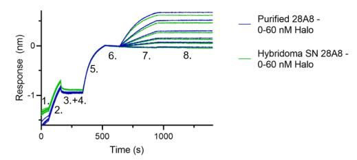
BLI binding kinetics of a purified and a hybridoma supernatant mouse IgG1 anti-Halo antibody to Halo-tag. A purified, monoclonal mouse IgG1 anti-Halo antibody (ChromoTek Halo antibody [28A8]) and a hybridoma supernatant, monoclonal mouse IgG1 anti-Halo antibody were immobilized using Nano-CaptureLigand mouse IgG1, Fc-specific VHH, biotinylated on FortéBio Streptavidin (SA) Biosensors and assayed with different concentrations of Halo-tag protein.
