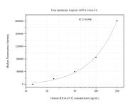
Cytometric bead array standard curve of MP51148-1, B3GALNT2 Monoclonal Matched Antibody Pair, PBS Only. Capture antibody: 60799-1-PBS. Detection antibody: 60799-2-PBS. Standard:Ag31400. Range: 12.5-200 ng/mL
