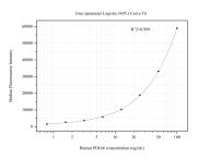
Cytometric bead array standard curve of MP50818-1, PDIA6 Monoclonal Matched Antibody Pair, PBS Only. Capture antibody: 66669-2-PBS. Detection antibody: 66669-3-PBS. Standard:Ag27608. Range: 0.781-100 ng/mL
