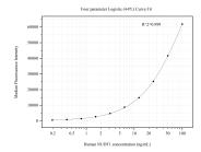
Cytometric bead array standard curve of MP50783-2, NUDT1 Monoclonal Matched Antibody Pair, PBS Only. Capture antibody: 67443-1-PBS. Detection antibody: 67443-4-PBS. Standard:Ag9802. Range: 0.195-100 ng/mL
