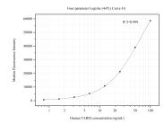
Cytometric bead array standard curve of MP50608-1, TARS2 Monoclonal Matched Antibody Pair, PBS Only. Capture antibody: 60449-1-PBS. Detection antibody: 60449-2-PBS. Standard:Ag7047. Range: 0.781-100 ng/mL
