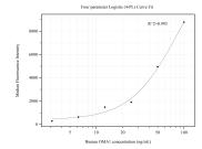
Cytometric bead array standard curve of MP50571-3, OMA1 Monoclonal Matched Antibody Pair, PBS Only. Capture antibody: 66572-1-PBS. Detection antibody: 67449-1-PBS. Standard:Ag11201. Range: 3.125-100 ng/mL
