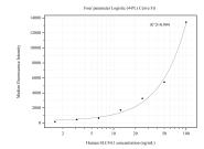
Cytometric bead array standard curve of MP50547-3, SLC 4A1 Monoclonal Matched Antibody Pair, PBS Only. Capture antibody: 66984-4-PBS. Detection antibody: 66984-3-PBS. Standard:Ag28058. Range: 1.563-100 ng/mL
