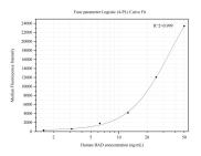
Cytometric bead array standard curve of MP50303-1, BAD Monoclonal Matched Antibody Pair, PBS Only. Capture antibody: 68902-1-PBS. Detection antibody: 68902-2-PBS. Standard:Ag34365. Range: 1.563-50 ng/mL
