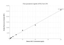
Cytometric bead array standard curve of MP01789-1, ASIC 1 Recombinant Matched Antibody Pair, PBS Only. Capture antibody: 85089-1-PBS. Detection antibody: 85089-3-PBS. Standard: Ag25941. Range: 0.313-40 ng/mL
