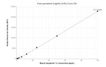
Cytometric bead array standard curve of MP01498-1, Semaphorin 7A Recombinant Matched Antibody Pair, PBS Only. Capture antibody: 84682-2-PBS. Detection antibody: 84682-1-PBS. Standard: Eg2005. Range: 0.781-100 ng/mL
