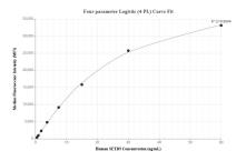
Cytometric bead array standard curve of MP01432-1, SETD5 Recombinant Matched Antibody Pair, PBS Only. Capture antibody: 84622-2-PBS. Detection antibody: 84622-1-PBS. Standard: Ag28929. Range: 0.469-60 ng/mL
