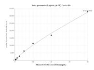
Cytometric bead array standard curve of MP01412-2, Cortactin Recombinant Matched Antibody Pair, PBS Only. Capture antibody: 84569-2-PBS. Detection antibody: 84569-1-PBS. Standard: Ag1940. Range: 0.313-40 ng/mL
