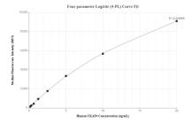
Cytometric bead array standard curve of MP01324-1, CKAP4 Recombinant Matched Antibody Pair, PBS Only. Capture antibody: 84485-1-PBS. Detection antibody: 84485-2-PBS. Standard: Ag10022. Range: 0.156-20 ng/mL
