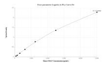
Sandwich ELISA standard curve of MP01320-4, Mouse CD147 Recombinant Matched Antibody Pair - PBS only. 84488-5-PBS was coated to a plate as the capture antibody and incubated with serial dilutions of standard Eg1530. 84488-4-PBS was HRP conjugated as the detection antibody. Range: 78.1-5000 pg/mL
