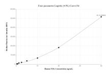
Cytometric bead array standard curve of MP01174-2, Noggin Recombinant Matched Antibody Pair, PBS Only. Capture antibody: 84283-1-PBS. Detection antibody: 84283-3-PBS. Standard: Ag32755. Range: 0.313-40 ng/mL
