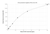
Cytometric bead array standard curve of MP01071-3, PCSK9 Recombinant Matched Antibody Pair, PBS Only. Capture antibody: 84172-4-PBS. Detection antibody: 84172-3-PBS. Standard: Eg0362. Range: 1.563-100 ng/mL
