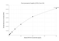
Cytometric bead array standard curve of MP00643-2, RNF216 Recombinant Matched Antibody Pair, PBS Only. Capture antibody: 83658-4-PBS. Detection antibody: 83658-1-PBS. Standard: Ag0238. Range: 0.625-80 ng/mL
