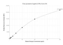
Cytometric bead array standard curve of MP00614-2, Glucagon Recombinant Matched Antibody Pair, PBS Only. Capture antibody: 83659-5-PBS. Detection antibody: 83659-4-PBS. Standard: Ag8677. Range: 0.313-40 ng/mL
