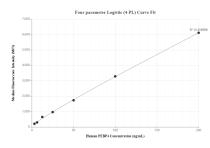
Cytometric bead array standard curve of MP00574-3, PEBP4 Recombinant Matched Antibody Pair, PBS Only. Capture antibody: 83589-3-PB5. Detection antibody: 83589-4-PB5. Standard: Ag9710. Range: 3.13-200 ng/mL
