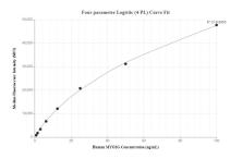
Cytometric bead array standard curve of MP00541-2, MYO1G Recombinant Matched Antibody Pair, PBS Only. Capture antibody: 83556-2-PBS. Detection antibody: 83556-1-PBS. Standard: Ag22698. Range: 0.78-100 ng/mL
