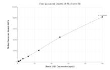
Cytometric bead array standard curve of MP00443-3, GNB3 Recombinant Matched Antibody Pair, PBS Only. Capture antibody: 83452-1-PBS. Detection antibody: 83452-2-PBS. Standard: Ag0127. Range: 0.78-100 ng/mL
