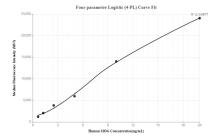
Cytometric bead array standard curve of MP00110-2, MOG Recombinant Matched Antibody Pair, PBS Only. Capture antibody: 83063-2-PBS. Detection antibody: 83063-4-PBS. Standard: Ag3273. Range: 0.625-20 ng/mL
