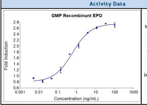
GMP Recombinant human EPO (HZ-1168-GMP) stimulates dose-dependent proliferation of the TF-1 human erythroleukemic indicator cell line. Cell number was quantitatively assessed by PrestoBlue® Cell Viability Reagent. TF-1 cells were treated with increasing concentrations of recombinant EPO for 72 hours. The EC50 was determined using a 4-parameter non-linear
