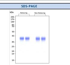
Purity of GMP-grade recombinant human EPO was determined by SDS- polyacrylamide gel electrophoresis. The protein was resolved in an SDS- polyacrylamide gel in reducing and non-reducing conditions and stained using Coomassie blue.
