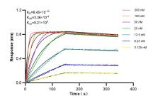
Biolayer interferometry (BLI) kinetic assays of 98151-1-RR against Human CD122/IL-2RB were performed. The affinity constant is 0.645 nM.
