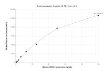
Cytometric bead array standard curve of MP01893-2, GREB1 Recombinant Matched Antibody Pair, PBS Only. Capture antibody: 85189-2-PBS. Detection antibody: 85189-1-PBS. Standard: Ag29908. Range: 0.781-100 ng/mL
