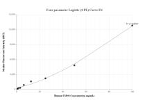
Cytometric bead array standard curve of MP01703-2, USP33 Recombinant Matched Antibody Pair, PBS Only. Capture antibody: 84958-2-PBS. Detection antibody: 84958-1-PBS. Standard: Ag14268. Range: 0.781-100 ng/mL.
