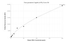
Cytometric bead array standard curve of MP01644-1, CHKA Recombinant Matched Antibody Pair, PBS Only. Capture antibody: 84881-1-PBS. Detection antibody: 84881-3-PBS. Standard: Ag4761. Range: 1.563-200 ng/mL
