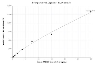
Cytometric bead array standard curve of MP01399-2, RAD51C Recombinant Matched Antibody Pair, PBS Only. Capture antibody: 84537-1-PBS. Detection antibody: 84537-3-PBS. Standard: Ag35070. Range: 0.469-60 ng/mL.
