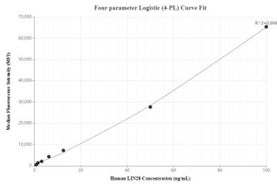
Cytometric bead array standard curve of MP00699-2, LIN28A Recombinant Matched Antibody Pair, PBS Only. Capture antibody: 83748-3-PBS. Detection antibody: 83748-1-PBS. Standard: Ag2312. Range: 0.78-100 ng/mL
