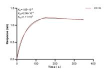
Biolayer interferometry (BLI) kinetic assay of 83634-3-PBS against Human OPTN was performed. The affinity constant is 1.85 nM.
