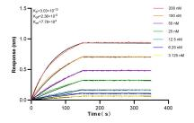
Biolayer interferometry (BLI) kinetic assays of 83254-1-RR against Mouse CD19 were performed. The affinity constant is 0.303 nM.
