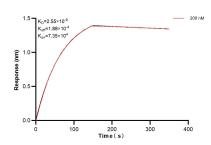
Biolayer interferometry (BLI) kinetic assay of 83185-4-PBS against Human Hemoglobin Alpha was performed. The affinity constant is 2.55 nM.
