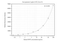
Cytometric bead array standard curve of MP50313-1, SENP1 Monoclonal Matched Antibody Pair, PBS Only. Capture antibody: 68907-1-PBS. Detection antibody: 68907-2-PBS. Standard:Ag18708. Range: 0.391-100 ng/mL.
