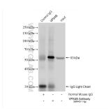
IP result of anti-VPS48 (IP:68443-1-Ig, 4ug; Detection:68443-1-Ig 1:4000) with HeLa cells lysate 1560 ug. This data was developed using the same antibody clone with 68443-1-PBS in a different storage buffer formulation.
