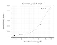
Cytometric bead array standard curve of MP50531-2, DDT Monoclonal Matched Antibody Pair, PBS Only. Capture antibody: 68314-5-PBS. Detection antibody: 68314-4-PBS. Standard:Ag3065. Range: 0.781-100 ng/mL
