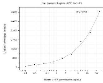
Cytometric bead array standard curve of MP50686-4, DHFR Monoclonal Matched Antibody Pair, PBS Only. Capture antibody: 68274-8-PBS. Detection antibody: 68274-7-PBS. Standard:Ag7318. Range: 0.098-25 ng/mL.
