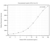
Sandwich ELISA standard curve of MP50052-2, SOD1 Monoclonal Matched Antibody Pair - PBS only. 67480-4-PBS was coated to a plate as the capture antibody and inc4bated with serial dilutions of standard Ag28553. 67480-3-PBS was biotinylated as the detection antibody. Range: 0.156-10 ng/mL
