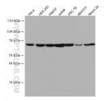
Various lysates were subjected to SDS PAGE followed by western blot with 67420-1-1g (RBM39 antibody) at dilution of 1:2500 incubated at room temperature for 1.5 hours.
