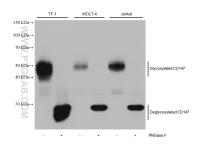
Untreated and PNGase F-treated lysates of TF-1 cells, MOLT-4 cells, Jurkat cells were subjected to SDS PACE followed by western blot with 66443-1 [g (CD147 antibody) at dilution of 1:20000 incubated at room temperature for 1.5 hours. This data was developed using the same antibody clone with 66443-1-PBS in a different storage buffer formulation.
