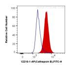
1X10^6 MCF-7 cells were intracellularly stained with 0.2 ug Anti-Human Cathepsin B (12216-1-AP) and Coralite®488-Conjugated AffiniPure Goat Anti-Rabbit IgG(H+L) at dilution 1:1000 (red), or 0.2 ug Control Antibody. Cells were fixed with 4% PFA and permeabilized with Flow Cytometry Perm Ruffer
