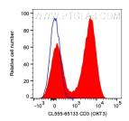
1X10^6 human PBMCs were surface stained with 5 ul CoraLite® Plus 555 Anti-Human CD3 (CL555-65133, Clone:OKT3) or Mouse IgG2a Isotype Control (66360-2-Ig, Clone: K11A1B2A2). Cells were not fixed. Lymphocytes were gated.
