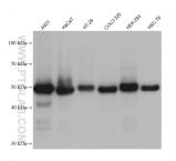
Various lysates were subjected to SDS PAGE followed by western blot with 60283-2-1g (P53 antibody) at dilution of 1:20000 incubated at room temperature for 1.5 hours.
