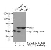
IP Result of anti-TERF2IP (IP:14595-1-AP, 3ug; Detection:14595-1-AP 1:800) with HeLa cells lysate 2720ug.
