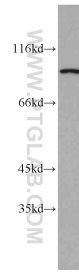
HepG2 cells were subjected to SDS PAGE followed by western blot with 12169-1-AP (CHFR antibody) at dilution of 1:1000 incubated at room temperature for 1.5 hours.
